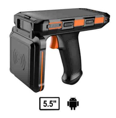
Intelligent devices with RFID shall satisfy industrial projects with reading distance up to 18 meters by pistol grip.
